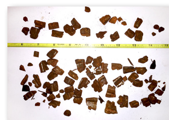
Slip debris from 5-1/2" TOMCAT
