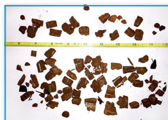
Slip debris from 5-1/2" TOMCAT
